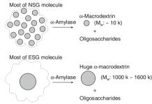
It has been shown that enzymatically-synthesized glycogen (ESG) has similar structural and physicochemical properties to natural source glycogen (NSG). However, hydrolysis of glycogens with an excess amount of alpha-amylase suggested a slight difference in the distribution of  $\alpha$ -1,6 linkages in ESG and NSG molecules.
